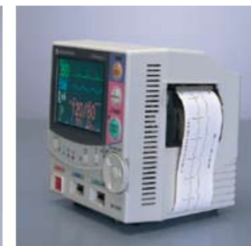
Recorder, RG-101W Built-in 2 ch thermal array recorder for recording waveforms and data, trend, and list
