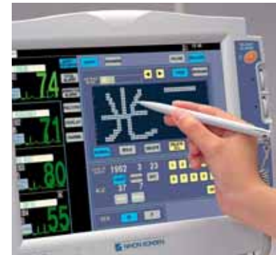
A touch panel and touch pen provide easy and quick operation. You can directly write the patient name on screen with the touch pen or finger. Any characters and figures can be displayed.
